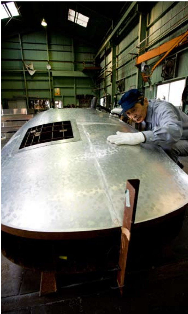
ON THE COVER: Yamashita Kogyosho Co., Ltd. sheet metal worker Jiro Kunimura fine tunes a part for a Shinkansen car using a hammer.
